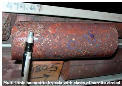
Multi-lithic haematite breccia with clasts of bornite circled
